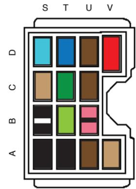
Temp. Gauge (engine connector location C-T)
