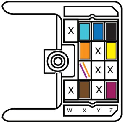
Tachometer (engine connector location A-X)
