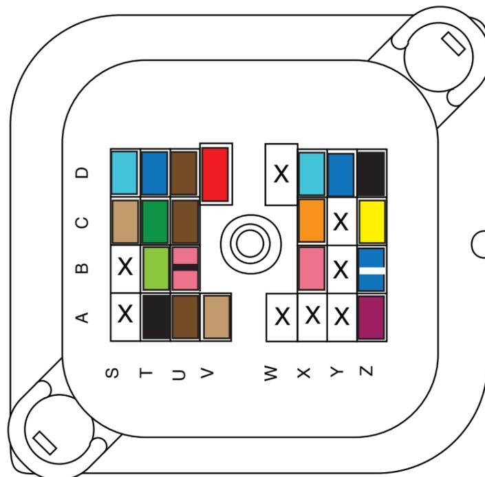
1968 - 1969 FUSE BLOCK BULKHEAD CONNECTOR
